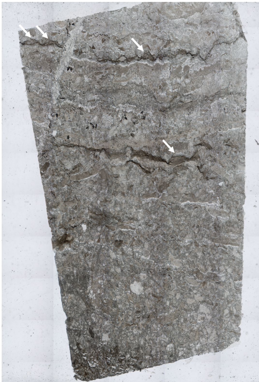
Figure S-3 Optical photomicrograph of thin section of Skillogalee Dolomite exhibiting silicified stromatolitic structures. Sample PM66-5. Organic-rich layers appear brown-grey in colour. Field of view is ~2 cm. Potential microdomical biogenic features, which may represent the incipient growth of microbial domes, are arrowed.
